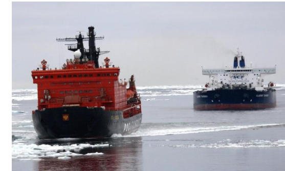
Atomic icebreaker «50 let Pobedy» is providing assistance on ice passage to «Vladimir Tikhonov» tanker at NSR
